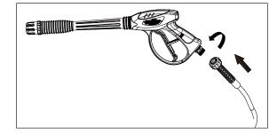
b. Attach the spray wand into spray gun. Tighten by hand.
