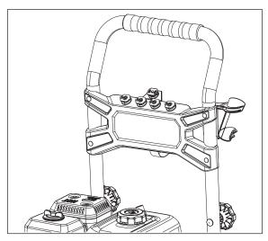
3. Attach the high pressure hose onto the hose hanger strap.
